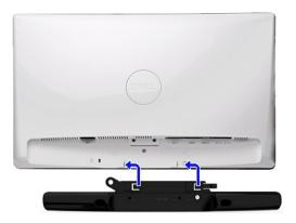
1. Working from the rear of the monitor, attach the Soundbar by aligning the two slots with the two tabs along the bottom rear of the monitor.
